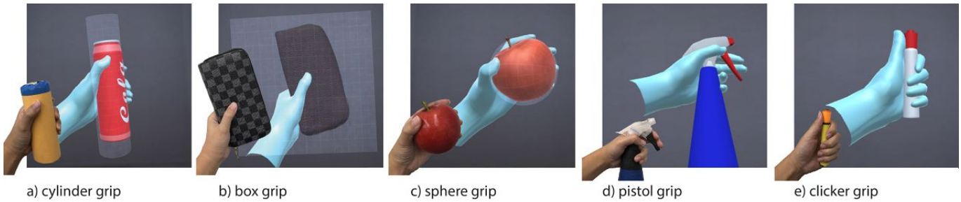
Figure 3. Tangible surfaces have three grip types: a) cylinder, b) box, and c) sphere. The estimated surfaces are shown in wireframes. Tangible tools have two grip types: d) pistol and e) clicker.
