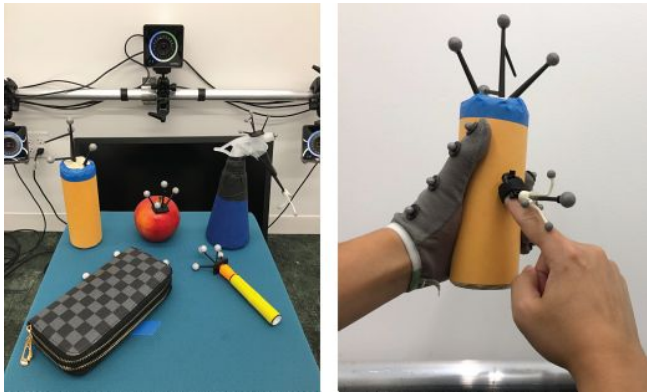
Figure 7. Left: The five objects are visualized through motion capture tracking. Right: The hands are tracked using marked gloves and the index finger is tracked with a single rigid body.
